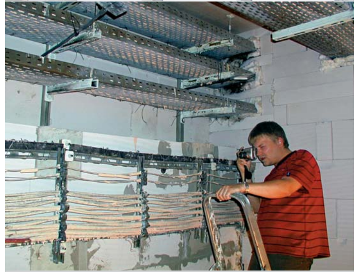
The fire-resistance test is being prepared. The installation system is assembled in the oven. After the test, results are documented by Petr Rojiček of Hilti Czech Republic.
